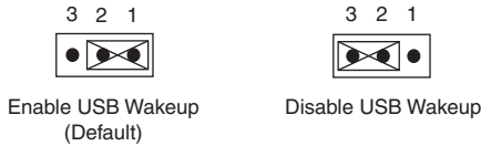
Figure B-3. Enable/Disable USB Wakeup Jumper: JPUSB1
