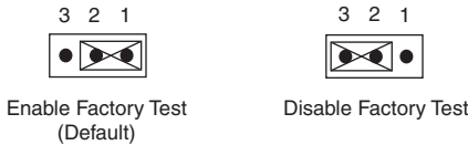
Figure B-4. Enable/Disable Factory Test Jumper: JPT1
